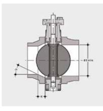
Before proceeding with the installation of the stubs, check that the bore of the fittings has sufficient clearance to allow the valve disk to open correctly. Also check the maximum coupling distance for the liner. Before proceeding with the installation of the FK valve, check that the bore of the stub allows the correct opening of the disk.
