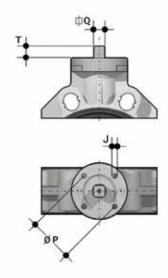
Actuator mounting flange The valve can be equipped with standard pneumatic or electric actuators and gearbox for heavy-duty operations, using a flange in PP-GR reproducing the drilling pattern provided for by standard ISO 5211.
