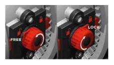
Rotate the button to the left, pointing the arrow on the open lock to unlock DUAL BLOCK®: the valve union nuts are free to rotate clockwise and counter-clockwise. Rotate the button to the right, pointing the arrow on the closed lock to lock DUAL BLOCK®: the valve union nuts are blocked in the desired position.
