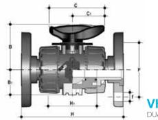
VKROAF DUAL BLOCK® regulating ball valve with ANSI B16.5 cl.150#FF fixed flange bore
