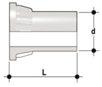
End connector in PVDF SDR 21 PN 16, long spigot, for butt welding
