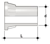
End connector in PVDF SDR 21 PN 16, long spigot, for butt welding
