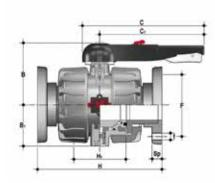
VKDOAF DUAL BLOCK <sup>®</sup> ball valve with ANSI B16.5 cl.150#FF fixed flanges.
