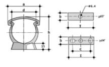
**ZAKM** Pipe clip for ASTM pipes in PP\*
