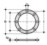
QHV/Y Flat gasket in EPDM for flanges according to DIN 2501, EN 1092, self-centring for flanges drilled PN 10/16
