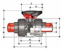
VKDIF/SHX DUAL BLOCK® 2-way ball valve with handle lock and STAINLESS steel threaded inserts for fastening, with female ends for butt welding, metric series
