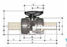
VKRBF DUAL BLOCK® regulating ball valve with long spigot male ends in PVDF for butt welding/ IR (CVDF)
