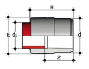
**RIF** Reducer: spigot (d), reduced socket for socket welding (d1)
