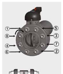
Before tightening the stud-bolts, it is advisable to open the disk in order to prevent damage to the seal. Tighten the stud-bolts in a uniform manner, in the order indicated in the figure, to the nominal operating torque value indicated in the table. The stud-bolts do not need to be excessively tightened in order to produce a perfect hydraulic seal. Overtightening could adversely affect the operating torque of the valve.
