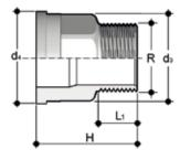
**Q/BRX** Union end in A316L STAINLESS steel with male BSP thread
