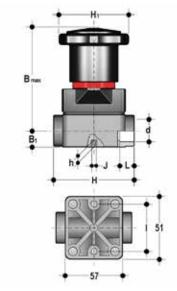
**CMIF** Compact diaphragm valve with female ends for socket welding, metric series
