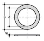
QHV/X Flat gasket in EPDM and FKM for flanges according to DIN 2501, EN 1092
